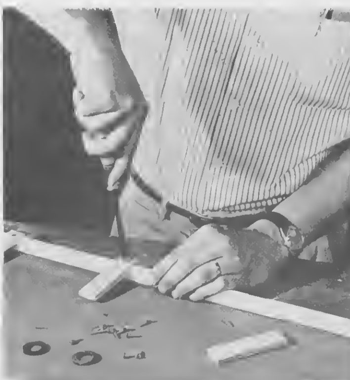
FASTENING PADDLES to the dowels looks tricky, but it isn't. A flat bed, the width of the paddle, is chiseled out of the dowel, and the paddles are glued or screwed in. MARAMENTO DI e remanan na e baranan ta muntra dificil, pero no ta. Un flat bed, hanchura di e rema ta worde sacá for di den e bara, y e remanan ta worde gelijm of geschroef aden.
